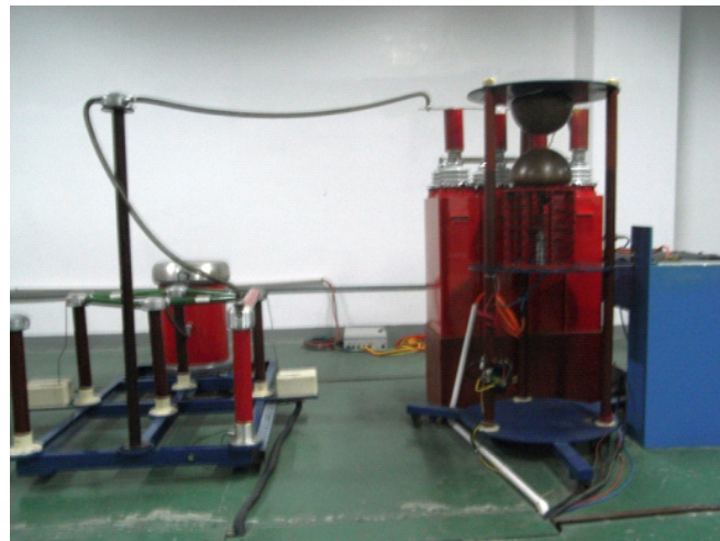
Figure 6: 8/20 \mu s impulse current generator
